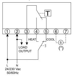
Terminal connections for heating or cooling systems.
