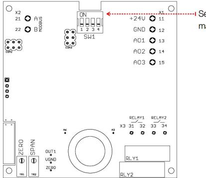
Set sensitivity to CALIBRATION max.10 minutes at fresh air
